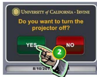
**i** Turning off the projector automatically sets room lights to "All On" and returns the touch-panel to the default screen.
