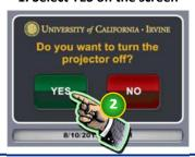
Turning off the projector automatically sets room lights to "All On" and returns the touch-panel to the default screen.
